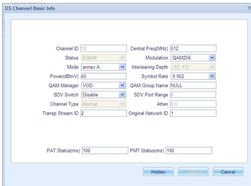
Figure 6.2-5 Advanced Configuration of Downstream Channel
