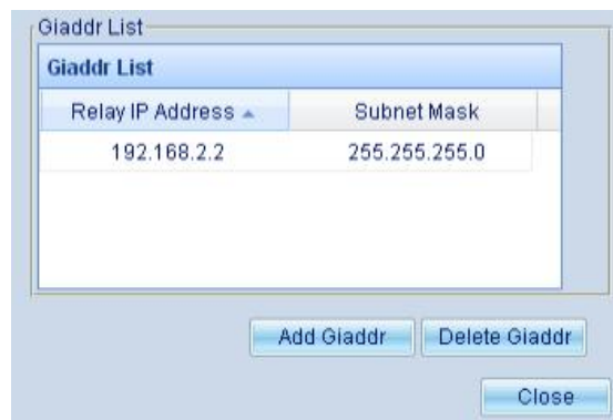
Figure 4.3-10 DHCP Relay Configuration Information
