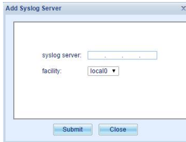
Figure 10.5-1 Adding a Syslog Server
