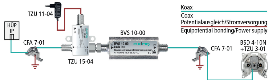
Fernspeisung BVS 10-00 am Verstärkereingang | Remote power supply BVS 10-00 at amplifier input
