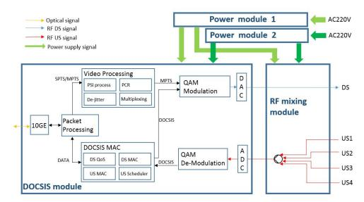
The main function is to converts data between the upper-layer network and the HFC network.
