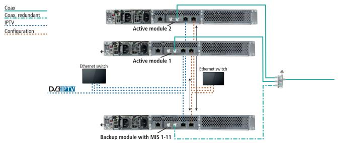
The backup module loads the configuration from the monitored modules and uses it in the event of an error.
