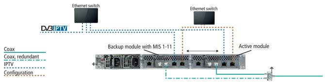
The illustration above shows module redundancy within an MIE. On the backup module, the output modulators are deactivated first. When switching to the backup unit, its output modulators become active and provide the output signal. The output modulators of the monitored module are deactivated in this case. A module with MIS 1-11 installed can monitor up to five other modules and serve as a backup module for these modules.
