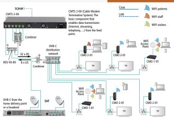
Any additional television supply that may be necessary or possible is provided via a cable connection, via a headend with SAT reception (Fig. above) or via an existing SAT IF installation.
