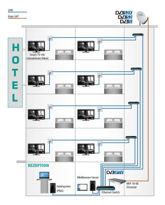
With the AXING encoders of the HKI series HDMI sources, e.g. external video sources, can be converted to IPTV (SPTS) and distributed in the same IP network.
